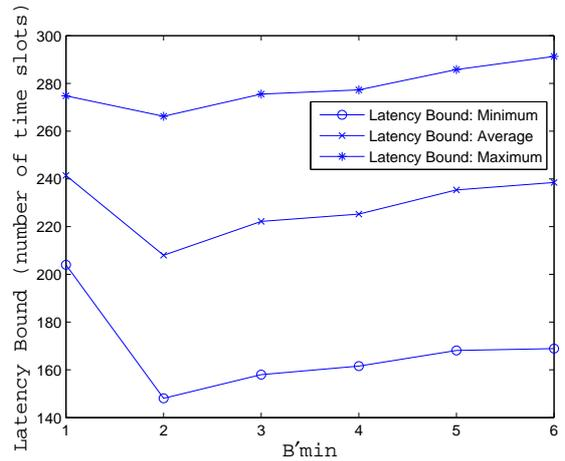
Figure 11: Effect of  $B'_{min}$  on Latency Bound
