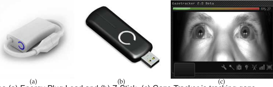
Fig. 6. Aeon Labs (a) Energy Plug Load and (b) Z-Stick. (c) Gaze Tracker is tracking gaze.
